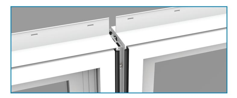
Snap in the interior and exterior mullion covers. This cover will snap and sit against both of the window units and cover up the mullion on both sides.
