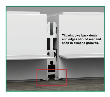
NOTE: Make sure the black gaskets are attached to the sides of the mullion before placing
