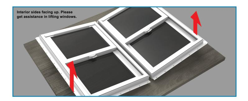
Align and insert the mullion in between the windows as the windows are slightly tilted up. There should be about 1/2" of space from the top and bottom of the window to the mullion (Mullions are pre-cut 1" shorter than height of windows). Then, as it is inserted, tilt the windows back down flush so it catches and snaps into the groove. The mullion piece should be slightly deeper inside the channel than the frame. Remove any excess sealant.
