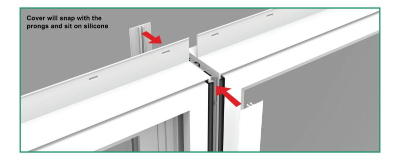
Completely seal the end conditions of the windows and the mullion with silicone. Do this for **both** the head (top) and under the sill (bottom) exposed mullion areas.
