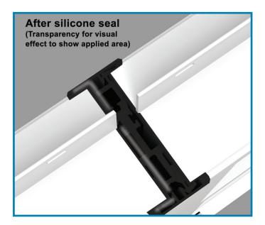
On the head (top) and sill (bottom), run a bead of silicone around the channel in preparation for SIKA tape. It should be a few inches out on each side from the sealed mullion.
