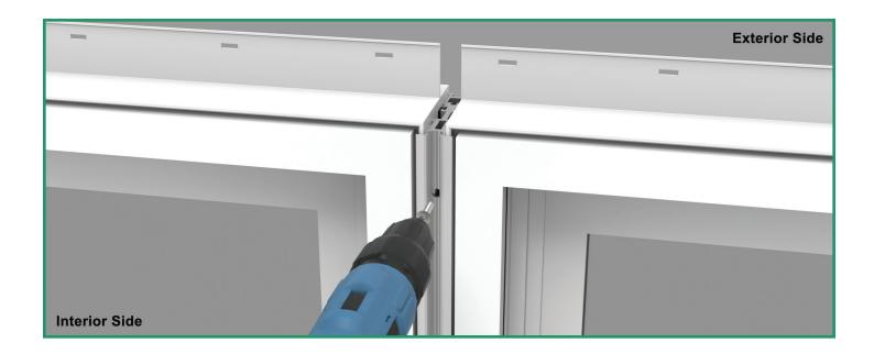
Optional, but recommended – In preparation for both cover pieces, place beads of silicone on each side of the mullion at the exterior and interior pockets.
