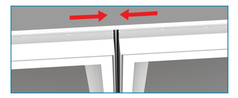
Center the mullion in between the windows in the groove – making sure that the mullion piece has a ½" space on the top and bottom. Each mullion piece will always be cut 1" shorter than the frame height. Also make sure the mullion has the gaskets on each side.
