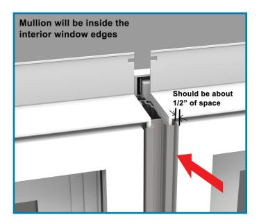
**Optional, but recommended** – In preparation for the interior cover piece, place beads of silicone on the mullion and interior cover pockets on the edges of the window.
