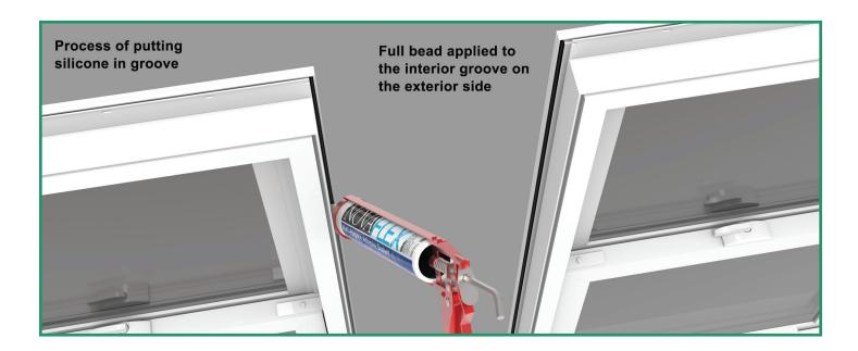
Butt the windows up next to each other so the exterior brick moulding from each window is touching in preparation for the mullion. There should be no gaps between the exterior window trim and a slight gap between the actual nail fins and frames.
