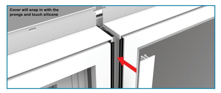
Completely seal the end conditions of the windows and the mullion with silicone. Do this for **both** the head (top) and under the sill (bottom) exposed mullion areas.
