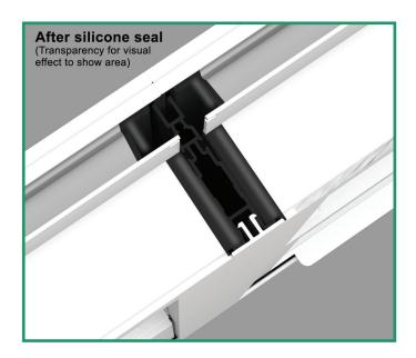
On the head (top), run a bead of silicone around J-channel in preparation for SIKA tape. It should be a few inches on each side from the mullion channel that was just sealed.
