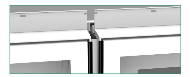
Snap in the interior mullion cover. This will be perfectly flush, edge to edge with both of the window units and cover up the mullion.
