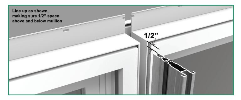
After being aligned properly, push the mullion piece in as far as you can. Use a rubber mallet and tap it the remainder of the way in. You may need a piece of wood to get in between the windows while using the mallet. The mullion piece should be slightly deeper inside the channel than the frame. The front prongs will go into the grooves with silicone.
