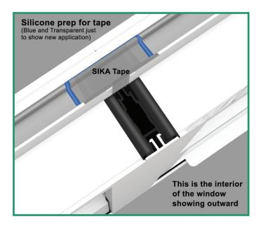
Press, tool and fully seal the silicone after the SIKA tape has been applied. Let the silicone cure before placing the windows, or the mullion may move and/or the windows may become misaligned.
