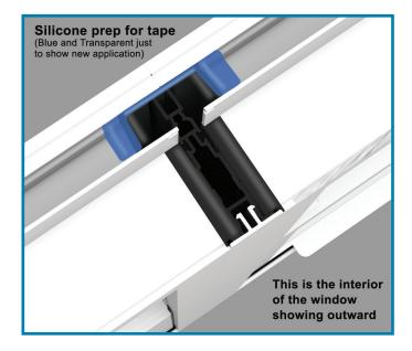
Apply the SIKA tape on the J-Channel pockets on head and sill exterior of nail fin to prevent anything from getting in the channel when siding is applied to the window. You are essentially creating a bridge between nail fins.
