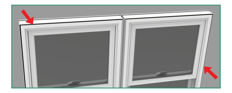
Place the ½" flange adaptor pieces in the silicone exterior accessory grooves around windows. **Do not** cut the adaptor apart in two pieces at the head or sill where windows meet. **You must make miter cuts to join the corners of the adaptors properly.**
