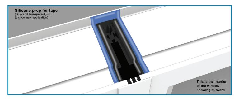
Place SIKA tape so it is flush with the  $\frac{1}{2}$ " flange adaptor and wrap it around the frame of the window covering the mullion. You are essentially creating a bridge between windows.
