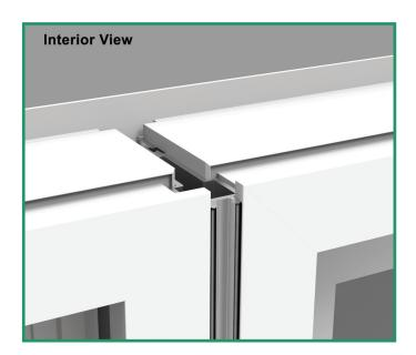
Snap in the interior and exterior mullion covers. Make any cuts necessary to line up the covers to fit in between the flange joints properly.
