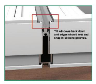
Locate the pre-drilled holes through the interior balance tracks of the windows inward towards the mullion. Use the screws (Teks #8 x 1/2" screws should be supplied in the kit) to fasten mullion to the windows. If a hung window, move sash up or remove to clear the balance and find all of the holes. If a casement, just open the window to see pre-drilled holes.
