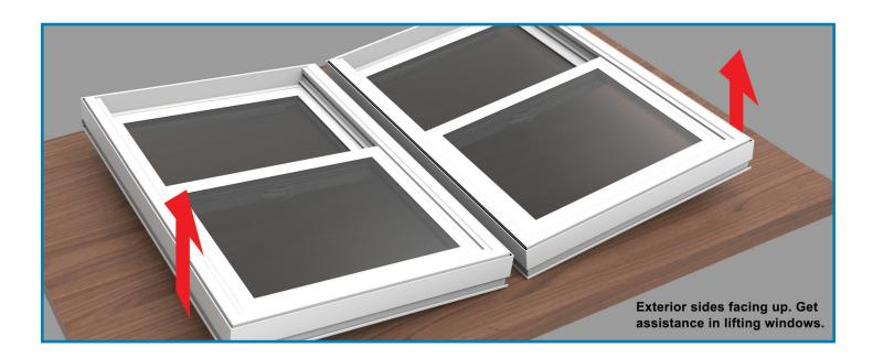
Insert the mullion in between the windows as the windows are slightly tilted up. Then as it is inserted, tilt the windows back down flush so it catches and snaps into the groove. The mullion should be flush with the frame on top and bottom (shorter than the top/bottom grooves).
