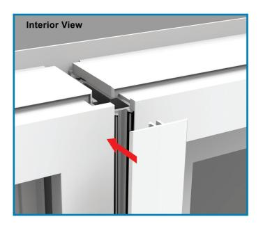
Completely seal the end conditions of the windows and the mullion with silicone. Do this for **both** the head (top) and under the sill (bottom) exposed mullion areas.
