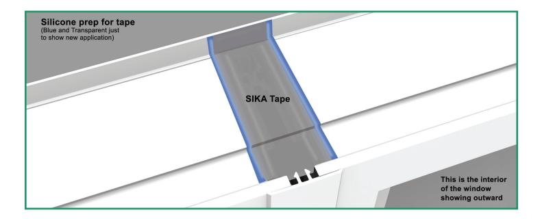
Press, tool and fully seal the silicone after the SIKA tape has been applied. Let the silicone cure before placing the windows, or the mullion may move and/or the windows may become misaligned.
