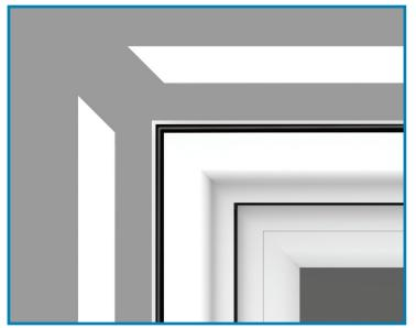
Apply a bead of silicone to the interior and exterior exposed sides of the mullion where the mullion covers will be snapped into.
