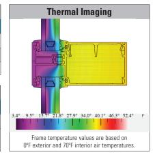
Test numbers are from the YWW 45 T system. YWW 40 test results should be similar.
