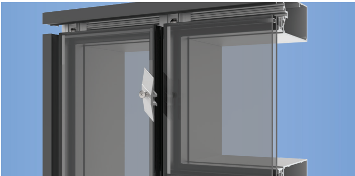
Rotating toggle locks are inserted on the vertical mullions to complete the unit installation. Silicone can now be applied.
