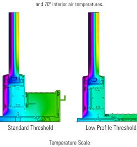
Frame temperature comparison values based on 0° exterior,
