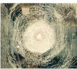
Building codes now call for Missile E protection for essential facilities (Risk Category 4) when the wind speed is 150 mph or greater. Missile E systems must withstand more than twice the impact energy compared to Missile D
