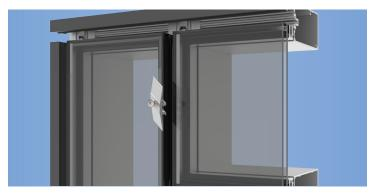
Rotating toggle locks are inserted on the vertical mullions to complete the unit installation. Silicone can now be applied.
