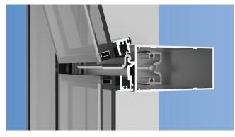
The panel cassette adaptor on the glass units interlock with the integral adaptor on the horizontal mullions.
