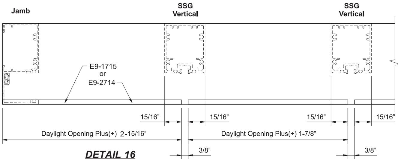
Exterior glass stops, E9-1715 for intermediate horizontals and E9-2714 for sills, may run continuous across SSG verticals. If so, a 3/8" expansion joint is required every 12 to 15 feet occurring at the centerline of a mullion.
