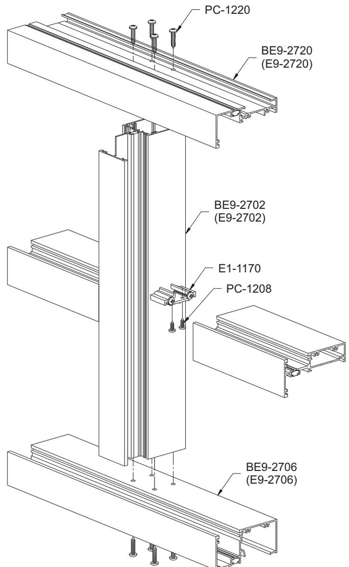
**Note:** Jambs for OG frames run full frame and do not require sealant at the ends.
