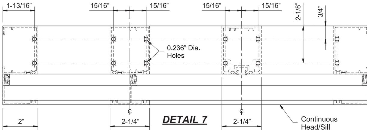
Continuous head and sill frames require weep holes at the sill:
