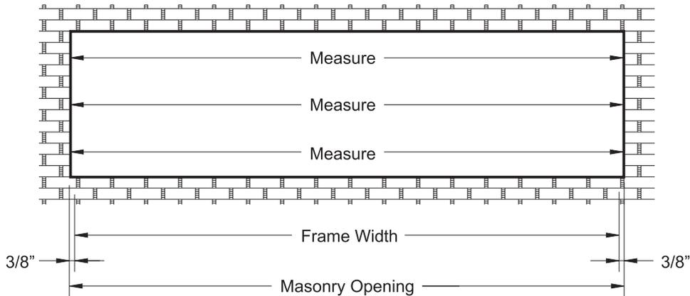
**Note:** Check opening for squareness of plumb at both ends, units must be installed in a true rectangle.
