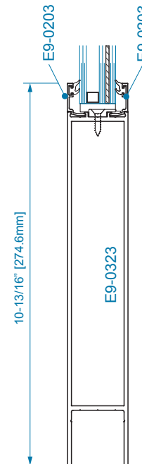
SECTION 3A 10" BOTTOM RAIL 1" DRY GLAZING
