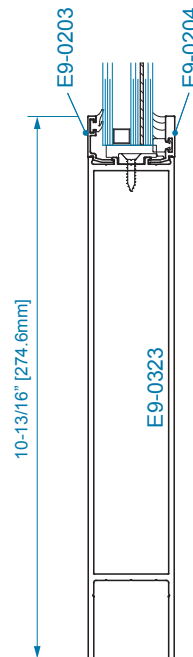
SECTION 3A 10" BOTTOM RAIL 1" WET GLAZING
