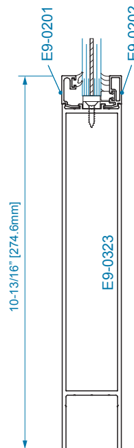
SECTION 3 10" BOTTOM RAIL 9/16" WET GLAZING
