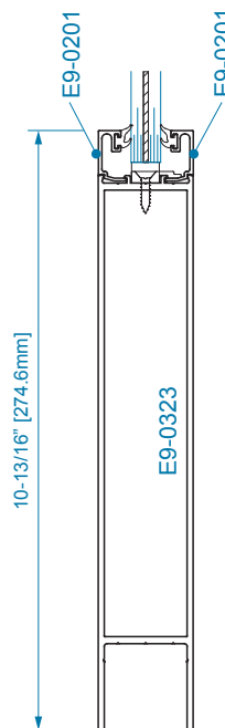
SECTION 3 10" BOTTOM RAIL 9/16" DRY GLAZING
