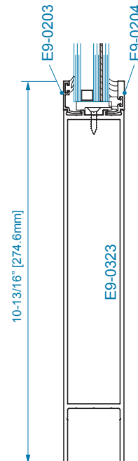
SECTION 3A 10" BOTTOM RAIL 1" WET GLAZING
