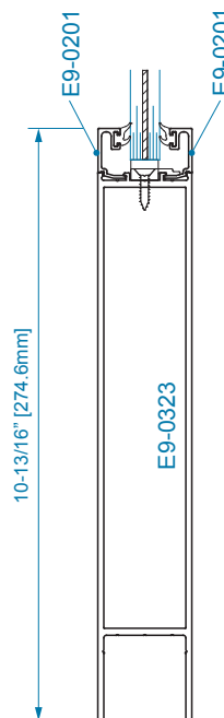
SECTION 3 10" BOTTOM RAIL 9/16" DRY GLAZING
