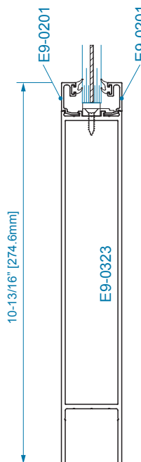
SECTION 3 10" BOTTOM RAIL 9/16" DRY GLAZING
